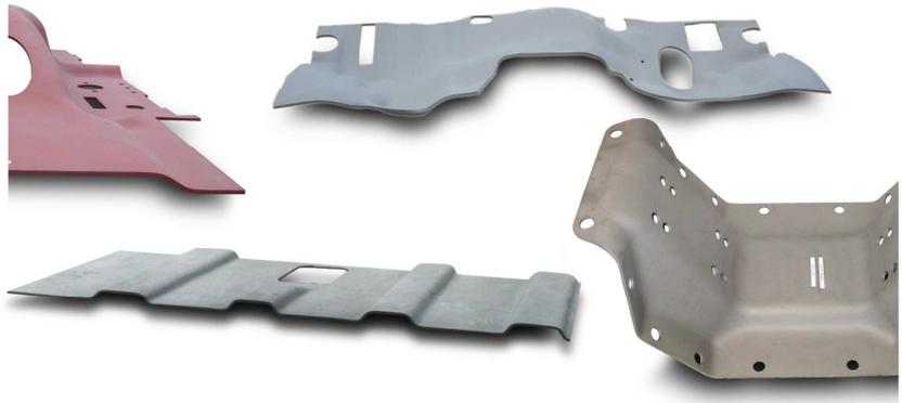
▲ Deform hot form, quench and temper armor plates to many different customers around the world.
