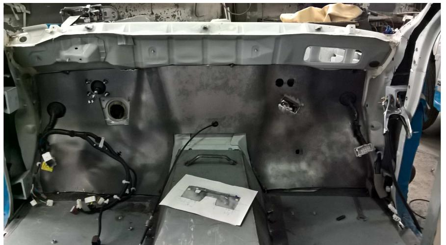
▲ Deform provides scanning at customer site and can then develop test models, bringing out adjustment (shape / hole pattern / outer contour) and finally produce tools. The picture shows a fire wall for mounting on a Nissan Patrol.
